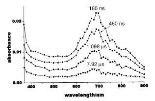
Fig. 5 Transient absorption spectra of an aqueous suspension of compound 2 incorporated in liposomes, recorded at different time intervals after a laser pulse excitation at 355 nm.
