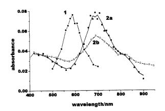
Fig. 4 Transient T–T absorption spectra of benzene solutions of derivatives 1 and 2. 1, compound 1 (flash photolysis experiment); 2a, compound 2 (flash photolysis experiment); 2b,  $5 \times 10^{-5}$  M benzene solution of compound 2 sensitised by  $1 \times 10^{-2}$  M naphthalene (pulse radiolysis experiment).
