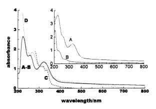
Fig. 1 Singlet ground state absorption spectra of the fullerene derivative 1 in benzene solution and incorporated in liposomes. A, compound 1 incorporated in liposomes; B, pure liposomes; A – B, difference spectrum; C, benzene solution of 1; D, thin solid layer of 1.
