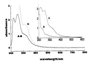
Fig. 2 Singlet ground state absorption spectra of the fullerene derivative 2 in benzene solution and incorporated in liposomes. A, compound 2 incorporated in liposomes; B, pure liposomes; A - B, difference spectrum; C, benzene solution of 2.
