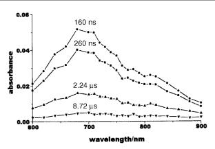
**Fig. 6** Transient absorption spectra of an aqueous suspension of compound **3** incorporated in liposomes, recorded at different time intervals after a laser pulse excitation at 355 nm.
