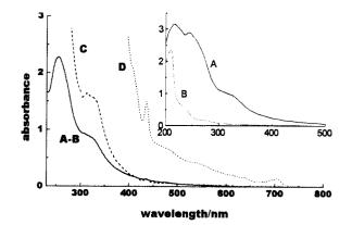
Fig. 3 Singlet ground state absorption spectra of the fullerene derivative 3 in benzene solution and incorporated in liposomes. A, compound 3 incorporated in liposomes; B, pure liposomes; A – B, difference spectrum; C and D, benzene solutions of 3 at concentrations of  $5 \times 10^{-4}$  and  $5 \times 10^{-5}$  M, respectively.
